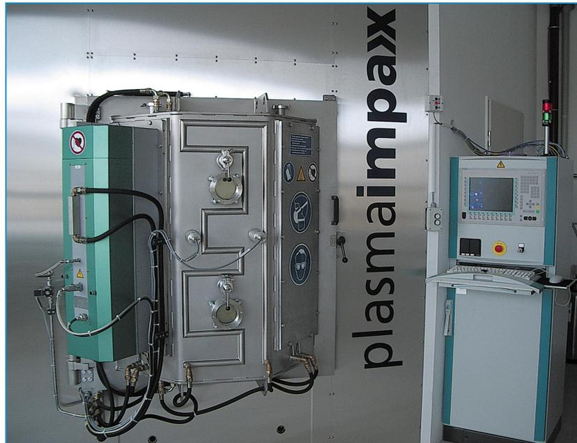
*Plasmaimpax coating system for deposition and ion treatments of implants and components for medical as well as automotive and engineering applications ■*
