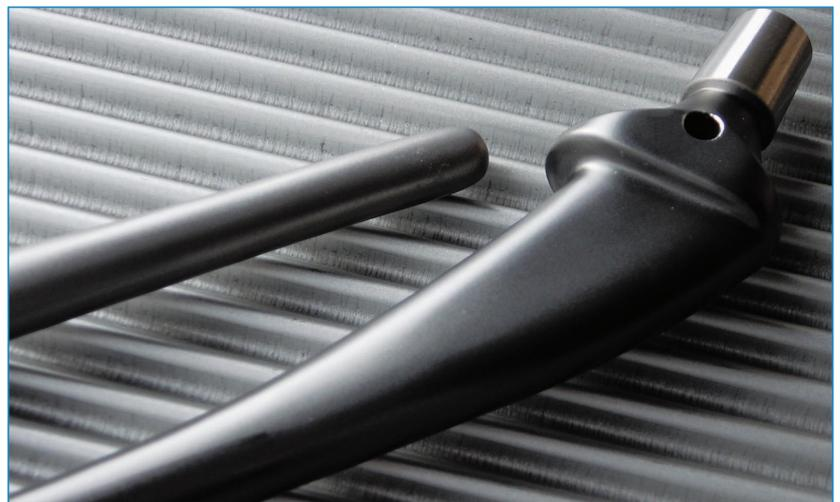
Low-friction and wear resistant DLC-coating (axyprotect®) on a titanium hip shaft ■
